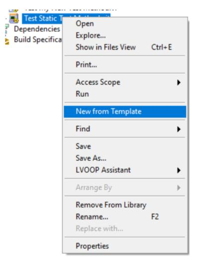
You can create test methods any way you like and you are free to delete the template methods if you choose to. It is important however that the connector pane uses the same pattern of terminals as the template and that the name of the vi starts with the word test.
