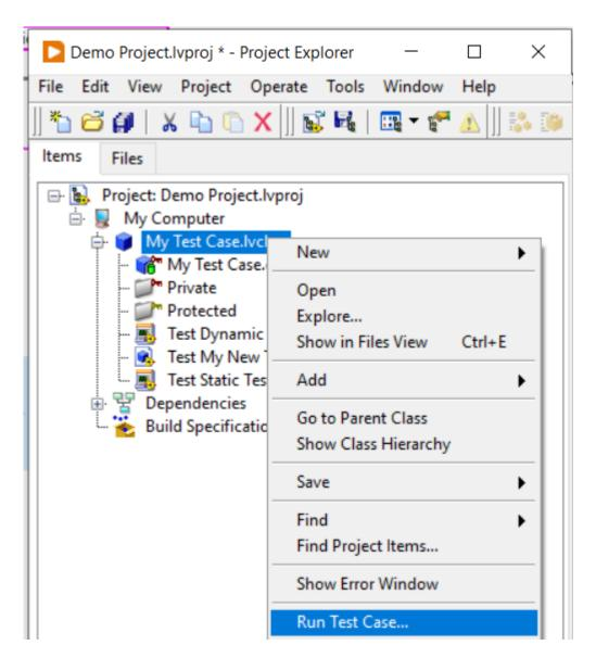
This will open the test execution user interface and run the test case. Alternatively you can also launch the user interface from the tools menu through the Tools > LUnit > LUnit UI... menu option. This will open the user interface and show all tests in the current project. As the test is run, the results are also shown as visual icons overlays in the project explorer.
