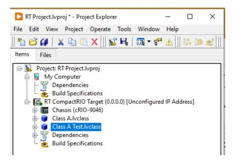
This works in principle, but LabVIEW will recompile the code for each test execution and is for this reason rather slow. This recompilation can be avoided by moving the test case to the My Computer target.
