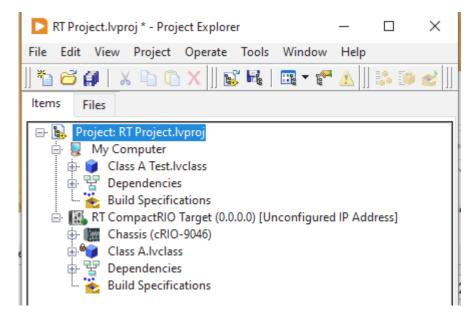
This speeds up the loading of the test as compilation is avoided, but it comes at the cost of locking the class under test. The lock occurs because the test case depends on the class under test, which is then loaded into two separate application instances.
