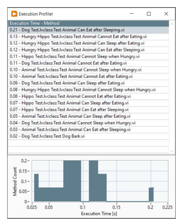
In the table, the execution time for the test and the test name are shown, ordered by test time. The histogram is useful to identify outliers and it is often these tests which have the biggest impact on the test execution time.
